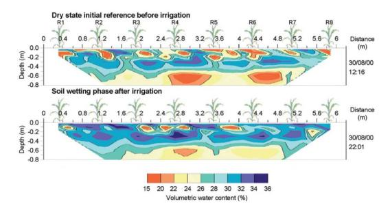
**Figure 15.** Changes in soil water content derived from ERT images, during irrigation of a corn crop (modified after *Michot et al.* [2003]). Thirty-two electrodes were placed at 0.2 m spacing along the ground surface. The images show changes in soil water content inferred from changes in resistivity.
