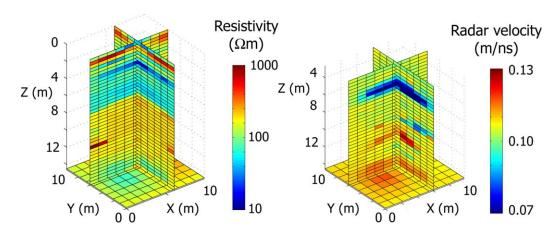
Figure 4. Example joint inversion of cross-well ERT and GPR data in the unsaturated zone of a sandstone aquifer (modified after *Linde et al.* [2006]). The 3-D volume contains regions where electrical conductivity (from cross-well ERT) and relative permittivity (from cross-well GPR) follow different joint relationships, which *Linde et al.* [2006] quantified to propose four lithological units.
