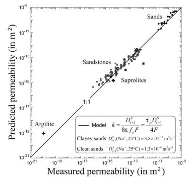
**Figure 7.** Comparison of permeability (*k*) modeled from SIP measurements of an electrical time constant  $(\tau_{\rho})$  or relaxation frequency  $(f_{\rho})$  and measured permeability (modified from *Revil* [2013]). Here  $D_{(+)}^{S}$  is the diffusion coefficient of cations in the Stern layer of the electrical double layer, and *F* is the formation factor.
