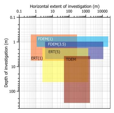
**Figure 5.** Comparison of horizontal and vertical survey scales typically achievable in 1 day by a two person field crew for ERT, FDEM, and TDEM. ERT(1) and ERT(5) refer to 1 and 5 m spaced electrode arrays, respectively. FDEM(1) and FDEM(3.5) refer to 1 m coil and 3.5 m coil instruments, respectively. For TDEM, we assume a 50 m loop sounding at multiple stations along a transect.
