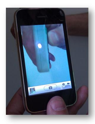
**Figure 1**. View of an IR LED being detected by an iPhone 3GS camera.
