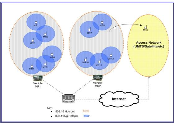
Figure 3: Model of the Mountain Rescue Network's infrastructure (adapted from [13])
