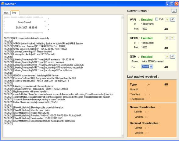
Figure 35 : The server application listening for packets and presenting the Log tab page
