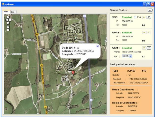
Figure 34 : The server application monitoring a "mission"
