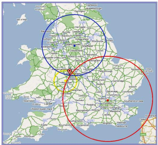
Figure 11 : Identify a unique location point based on the 2D equivalent procedure of the GPS.
