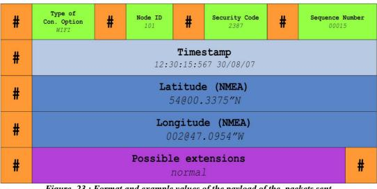
Figure 23 : Format and example values of the payload of the packets sent regardless of the connectivity option used
