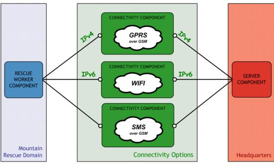
Figure  $1\overline{4}$ : System architecture focused on connectivity options
