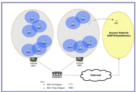
Figure 41 : Example of a Mountain Rescue Network's infrastructure (adapted from [8])
