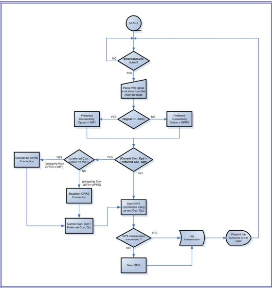
Figure 31 : Flow Chart of transmitting the GPS coordinates
