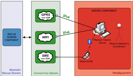
Figure 21 : System architecture focused on the Server Component
