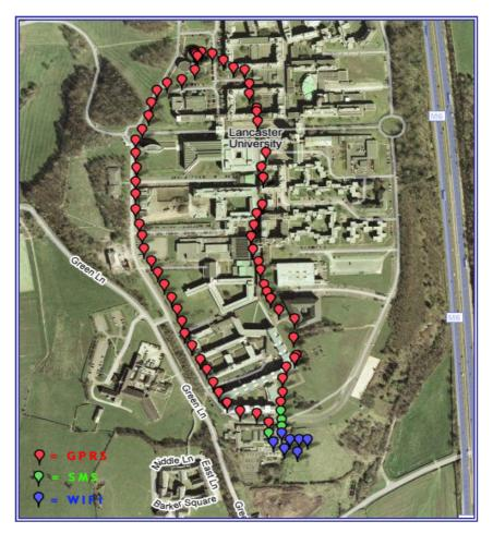
Figure 40 : Graphical representation of the GPS coordinates that were sent and the connectivity option that was used during our experiment<sup>35</sup>
