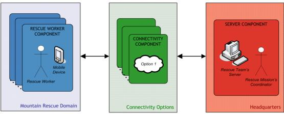
Figure 13 : High level system architecture overview
