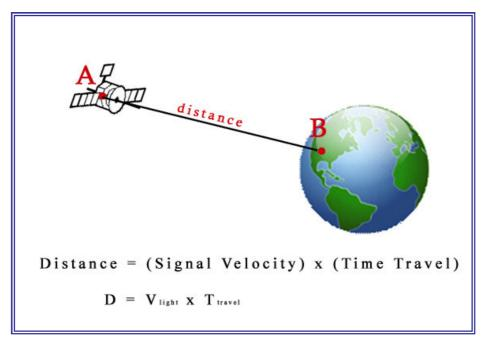
Figure 12 : Calculating the distance between a point with a known location (point A) and a point with unknown location (point B) by sending wave signals.
