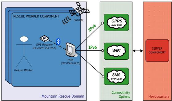
Figure 17: System architecture focused on the Rescue Worker Component
