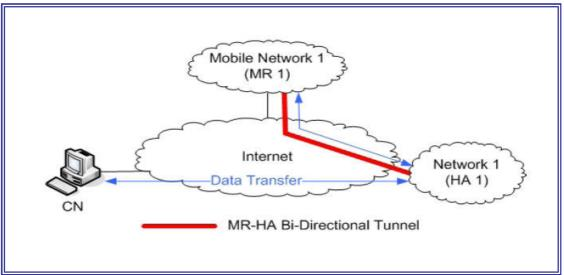
Figure 5: Communication imposed by the NEMO basic support protocol (adapted from [6])
