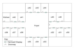
Figure 3 – layout of a specific region of the Computing Department in Infolab showing offices (c42, c43, etc.) and the Hermes2 displays situated adjacent to doorways
