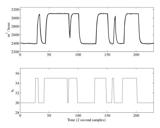
**Figure 1.3** Top: ventilation rate (m<sup>3</sup>/h) and response of the identified TF model (thick trace) Bottom: applied voltage to the control fan expressed as a percentage.
