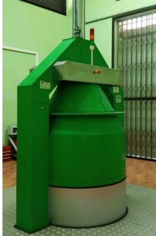
Figure 1 Self-contained Irradiator Category one (Model: Ob-Servo Ignis Research Gamma Irradiator, Manufacturer: Izotop Institute of Isotopes).
