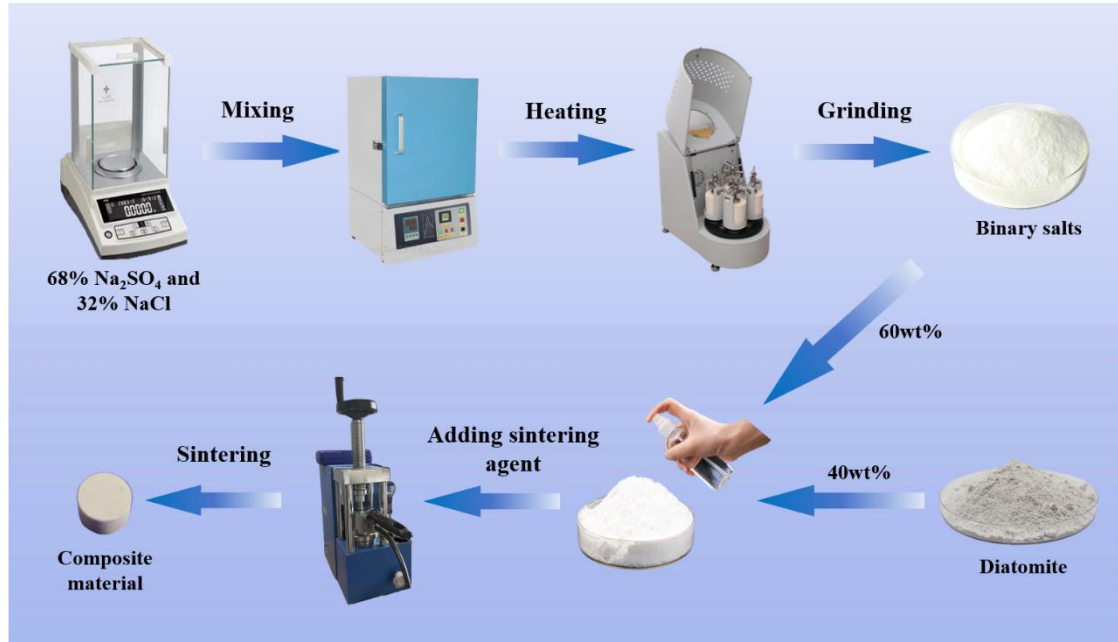
Fig. 1. Preparation process for the salt-diatomite composite phase change materials using cold sintering technique.
