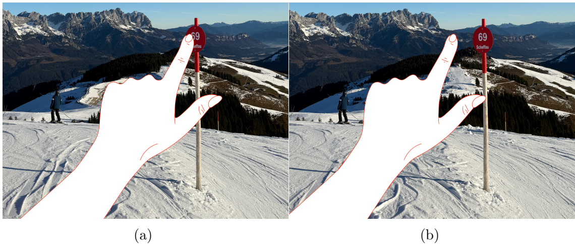
Figure 1.2: Visual representation of parallax during pointing. Because the same object is viewed from two different perspectives (left and right eye), an apparent displacement relative to the background occurs. a) When viewing from the left eye, the finger is perceived on the object. b) When viewing from the right eye, the finger is perceived next to the object.
