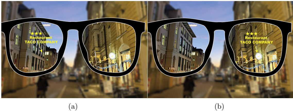
Figure 8.3: Conceptual Illustration Dominant Eye Aware AR Visual Layout. a) Label placement in the non-dominant eye (left eye). Content and label are misaligned. b) Label placement in accordance with the users' dominant eye (right eye). Label is aligned with content.
