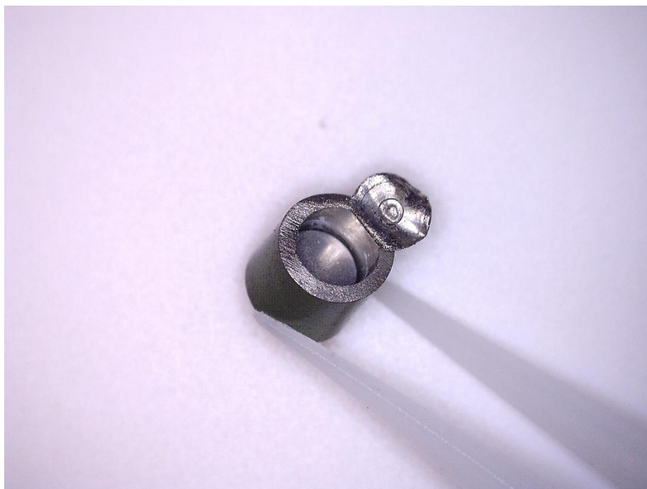
Fig. 4. 10: Crucible post-experiment (81.2 mol% RbF- 18.8 Mol% CeF 3 ) sanded open and inspected for corrosion.
