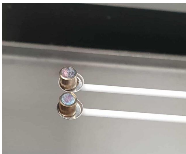
Fig. 3. 5: Sealed sample (below) and reference (above) DSC crucibles on horizontal Hitachi STA72000 sample holders post-experiment displaying minor oxidation on the outer surfaces.
