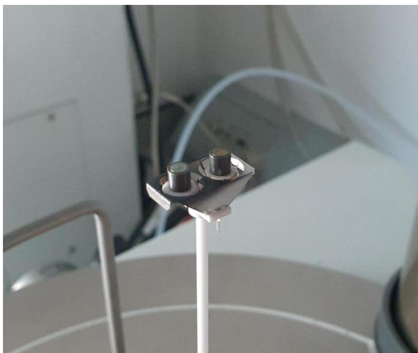
Fig. 4. 9: Sealed custom-made crucibles developed at Lancaster University NETZSCH STA 449 F3 Jupiter crucible holder with protective alumina disks post-run
