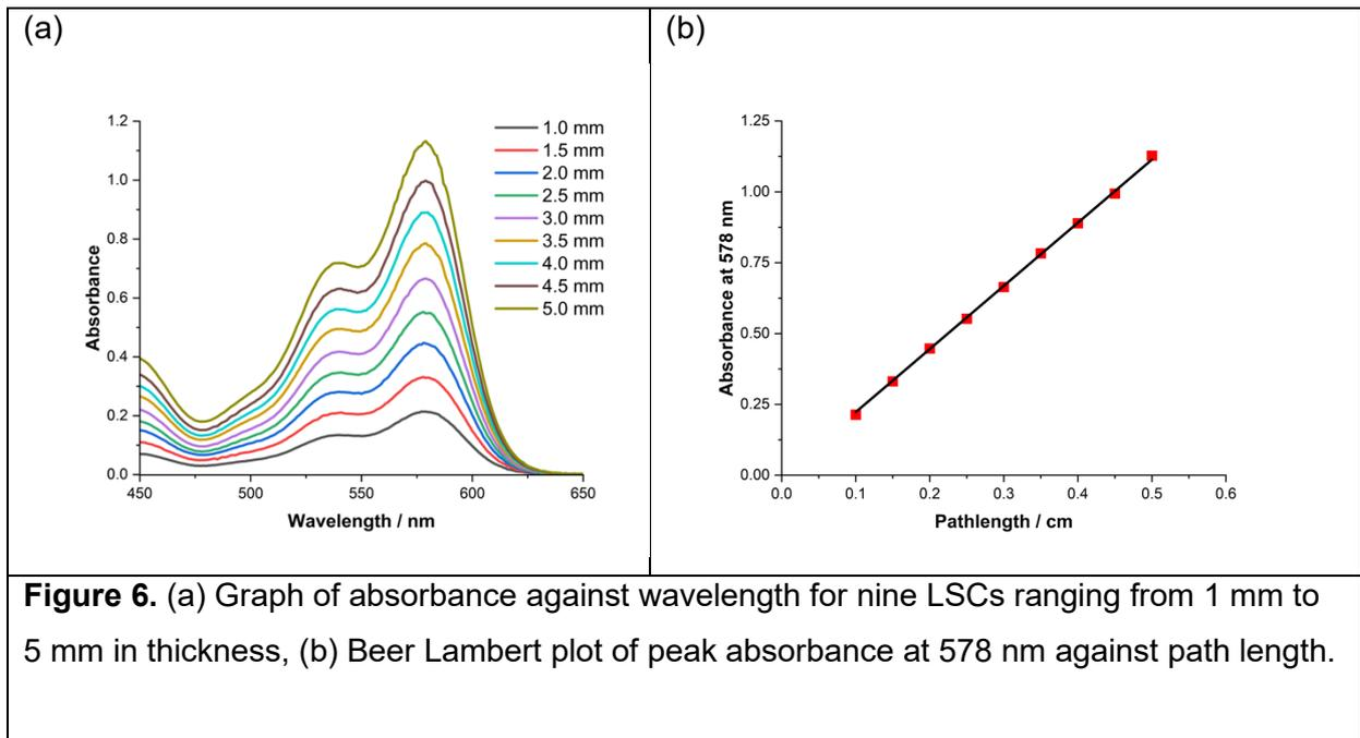
**Figure 6.** (a) Graph of absorbance against wavelength for nine LSCs ranging from 1 mm to 5 mm in thickness, (b) Beer Lambert plot of peak absorbance at 578 nm against path length.
