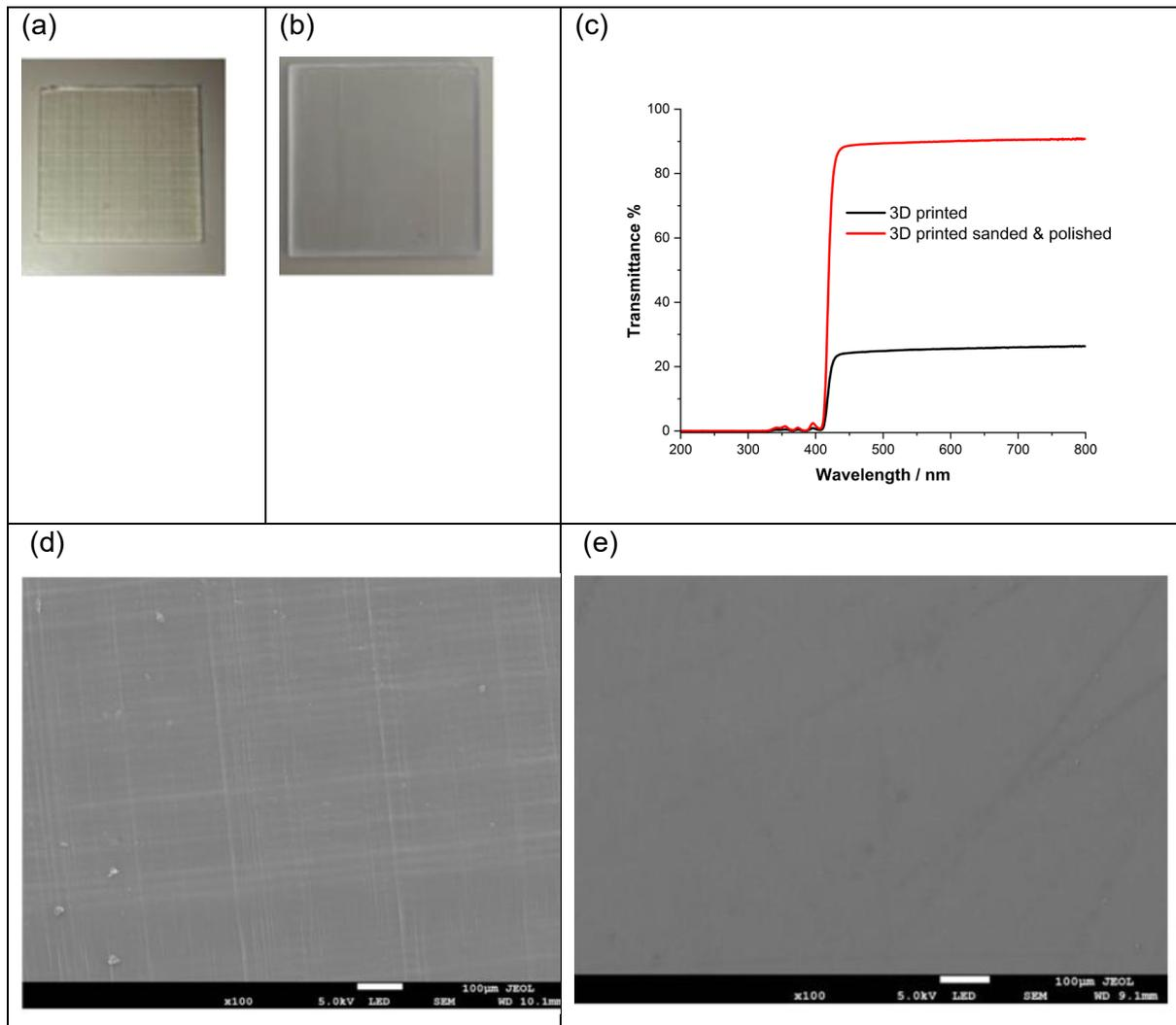
**Figure 3.** (a) Photo of a 3D printed blank LSC with no surface treatment, (b) Photo of a 3D printed blank LSC after sanding and polishing, (c) Graph of transmittance against wavelength showing the transparency improvement, (d) SEM image of a 3D printed blank LSC before surface treatment,  $\times 100$  magnification scale bar  $100\ \mu\text{m}$ , (e) SEM image of a 3D printed blank LSC after sanding and polishing  $\times 100$  magnification scale bar  $100\ \mu\text{m}$ .
