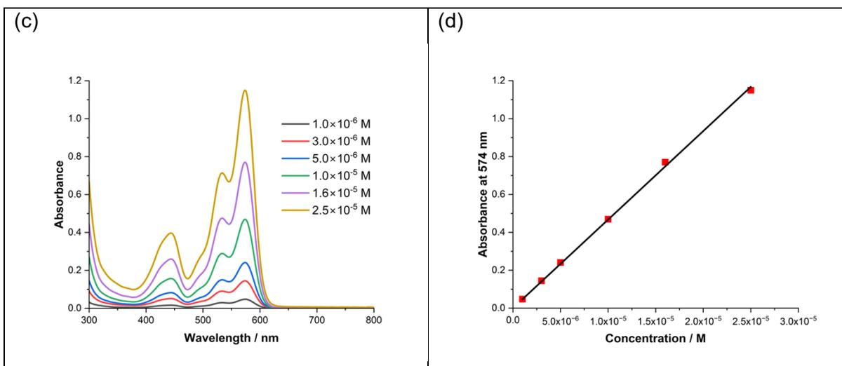
**Figure 2.** (a) Chemical Structure of Pe-Red used in this work. (b) Absorption and emission spectra of Pe-Red dissolved in toluene. (c) Absorption spectra for Pe-Red for six different concentrations (in toluene). (d) Beer-Lambert plot of concentration vs absorbance at a wavelength of 574 nm. The molar absorption coefficient (at 574 nm) is estimated to be  $46,704 \pm 109 \text{ M}^{-1} \text{ cm}^{-1}$ .
