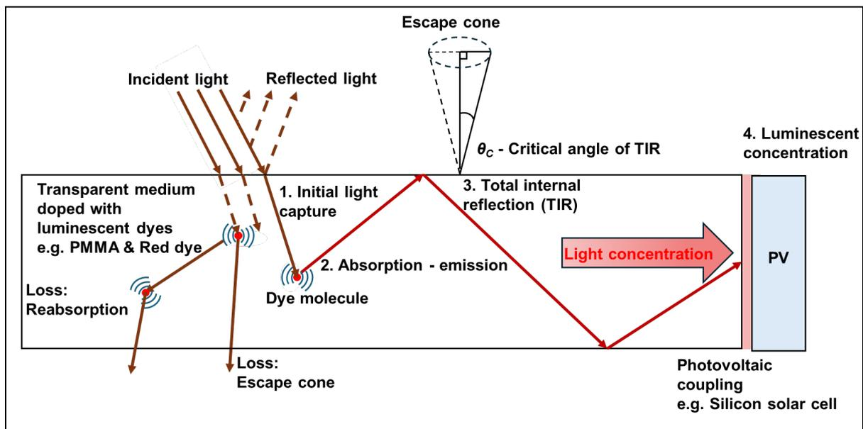
**Figure 1.** Schematic of the operation of a Luminescent Solar Concentrator (LSC). Light is incident through the front face of the LSC and is absorbed by a luminophore (1). After absorption the dye is excited and undergoes isotropic emission (2). A significant part of the emitted light is trapped via total internal reflection (TIR) (3) and directed to the edge of
