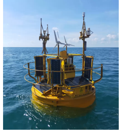
(c) Buoy-fitted wind LiDAR used at North Sea site. Courtesy of ZX Lidars.
