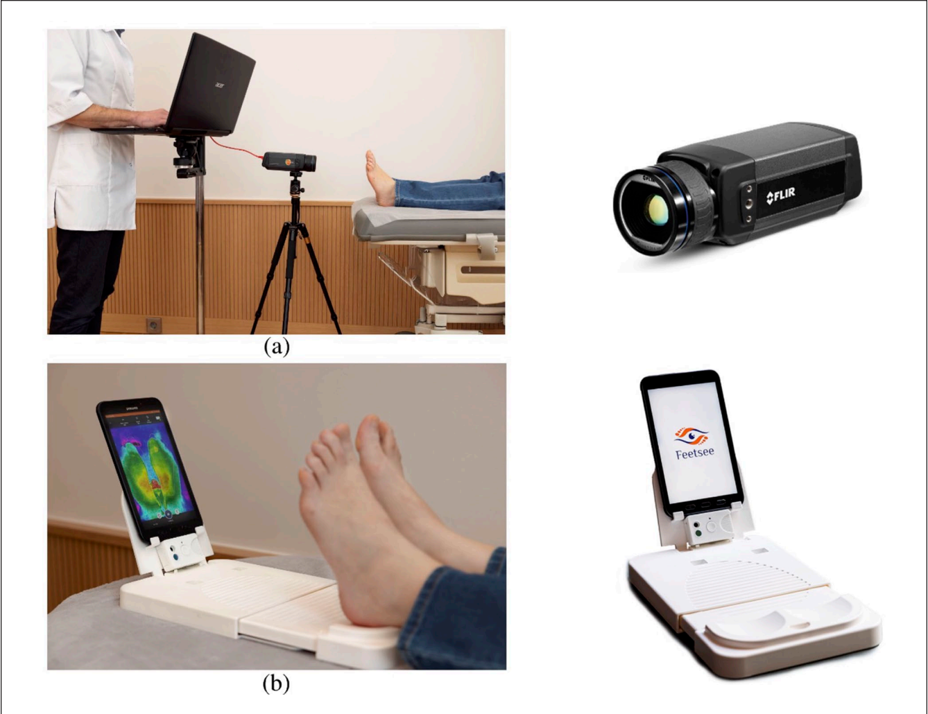
Figure 1. Thermal measurement experimental set-up with (a) RefCam and (b) InvCam device.
