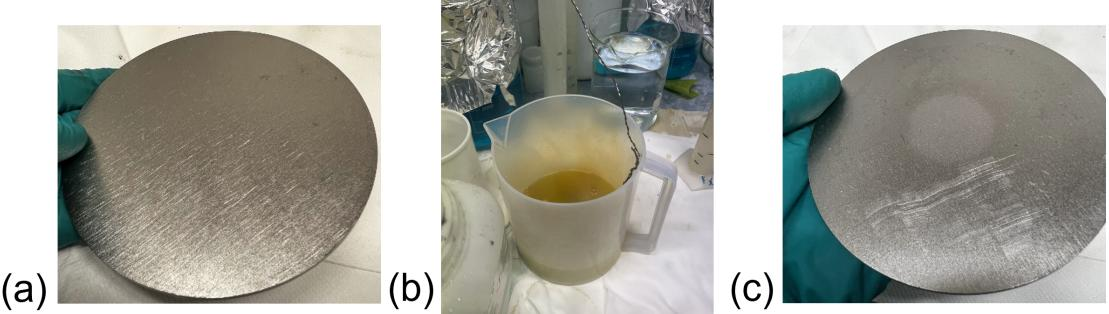
Figure 7.1: The BCP process for the bulk Nb disk: (a) un-polished disk, (b) disk submerged in the BCP solution, (c) post-polished disk. Image courtesy: E. Chyhyrynets (INFN).
