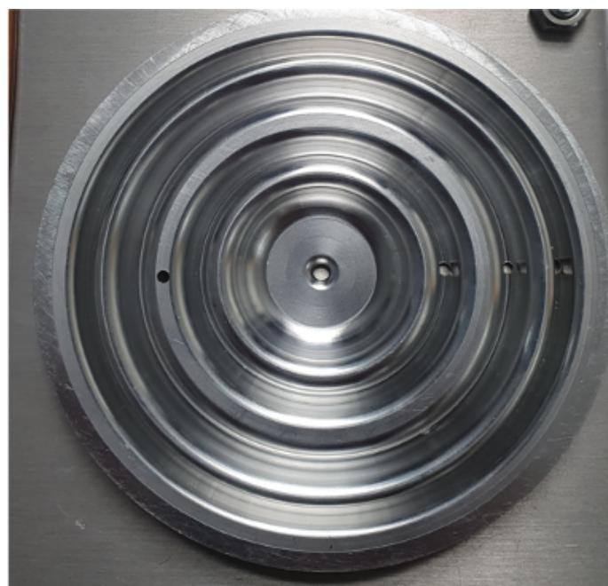
Figure 4.29: The manufactured bulk Nb Choke Cavity.
