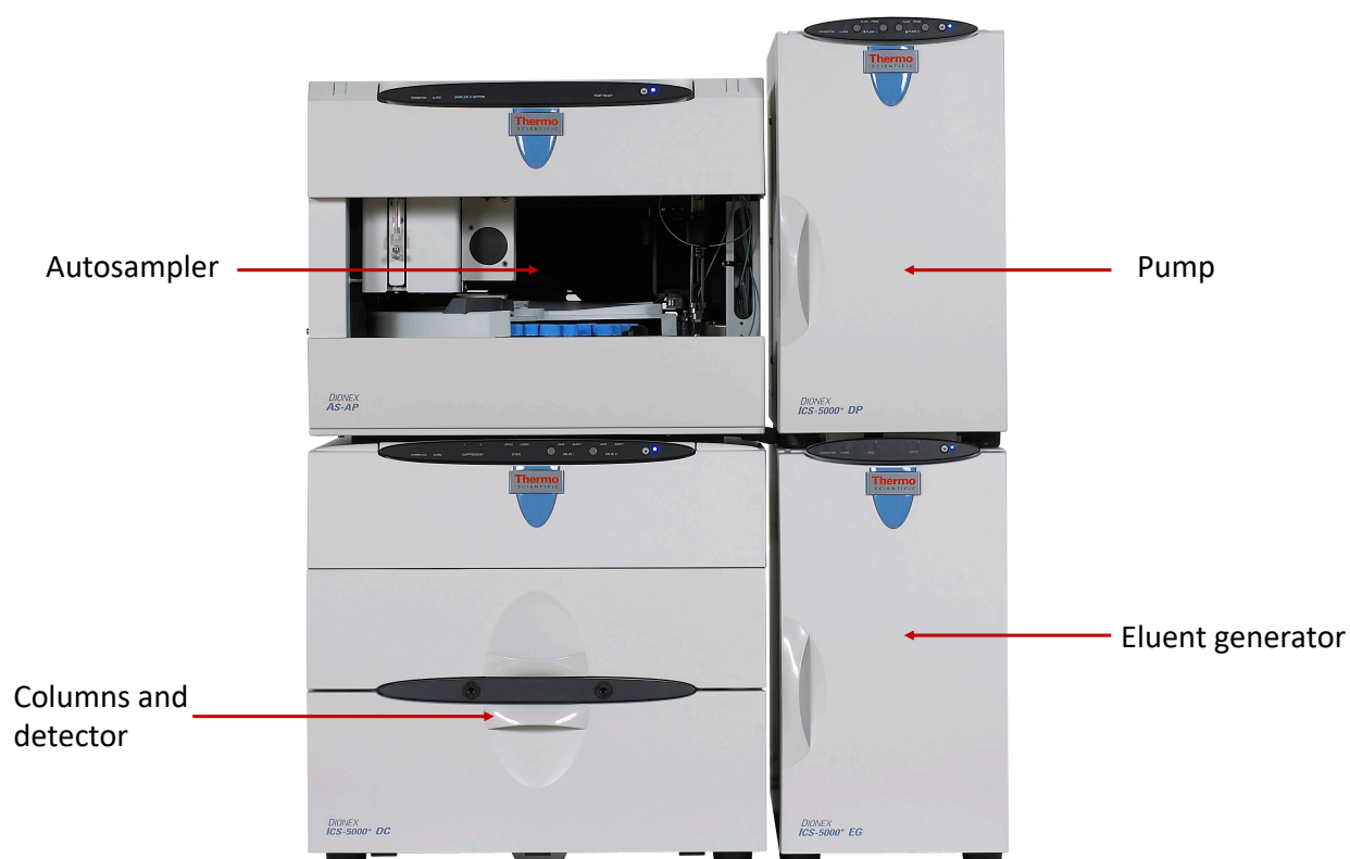
Figure 3-8: Ion chromatography instrument Thermo Scientific ICS 5000.
