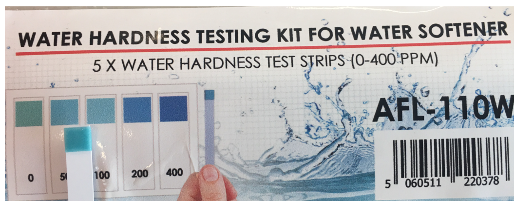
Figure 5-5: Strip-based kit for water hardness determination (FilterLogic).
