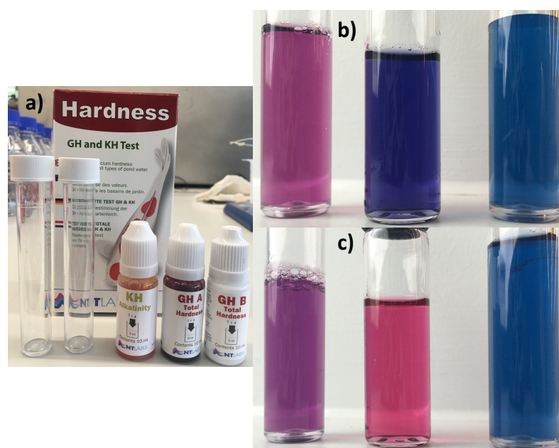
Figure 5-6: a) Titration-based kit for hardness water determination (£8.99 for kit allows analysis of up to 50 samples), b) soft water examination, c) hard water examination.
