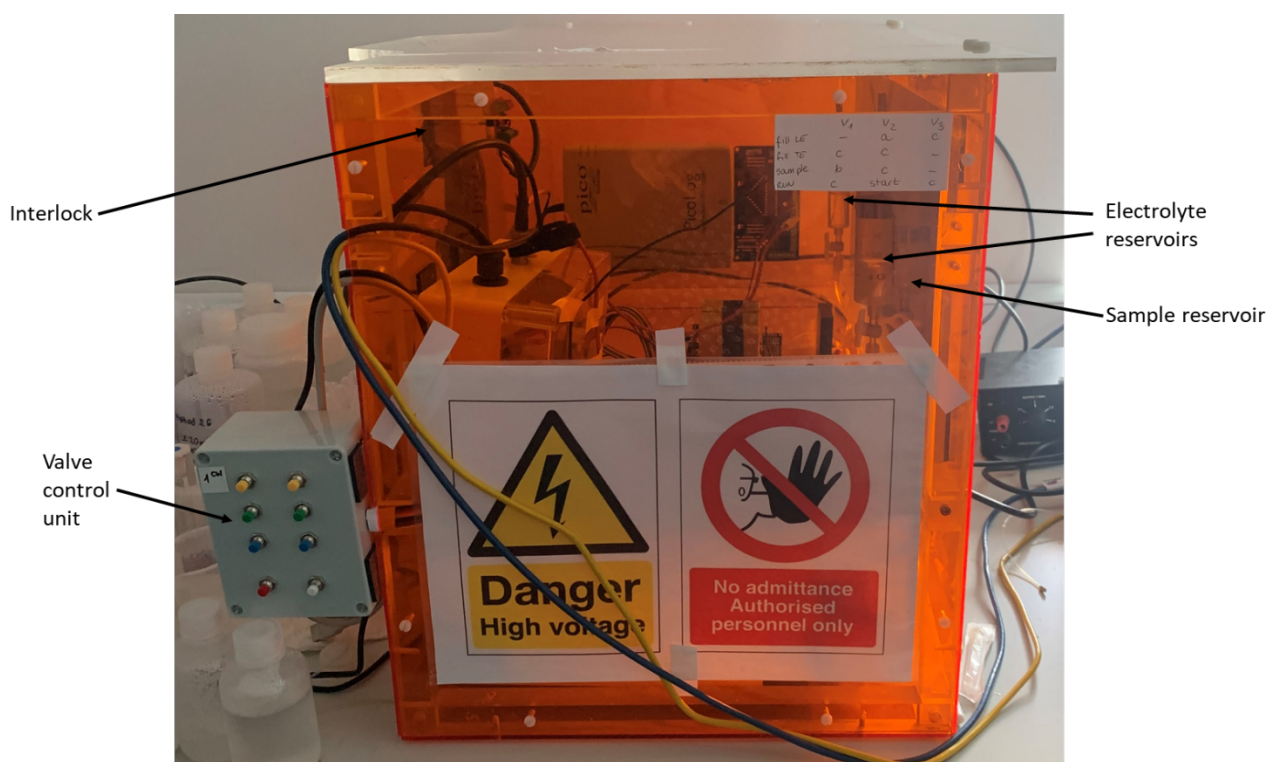
Figure 6-10: Instrument prototype in the safety box side view.
