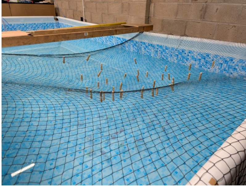
Figure 11 – Net overlay suspending artificial targets using wooden pegs and monofilament wire
