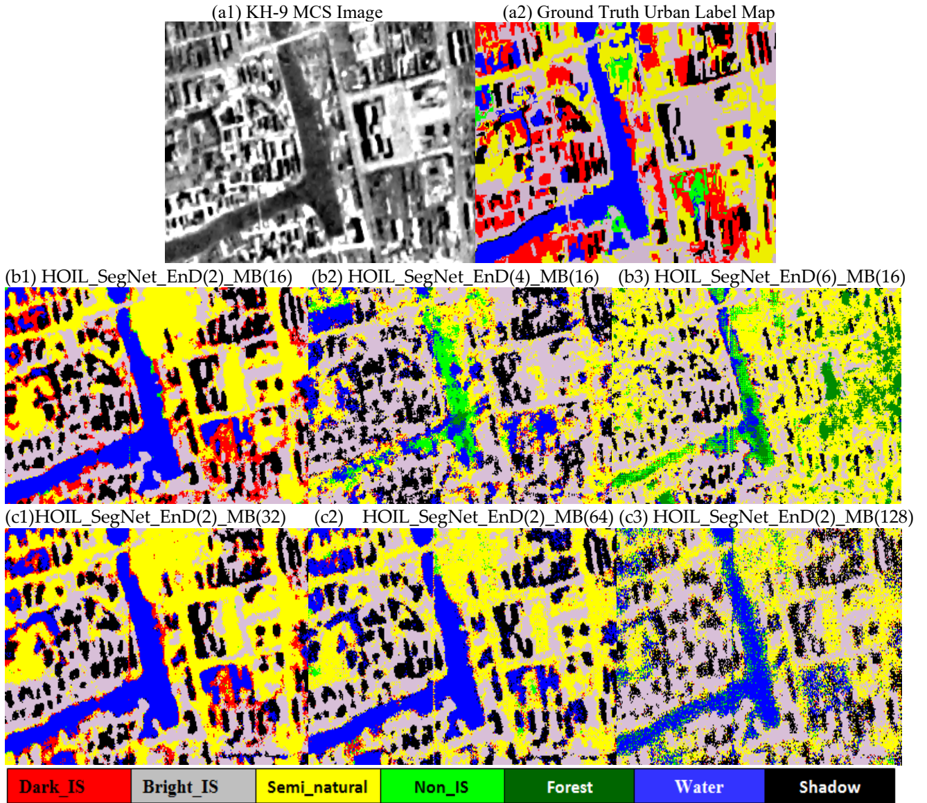
Fig.4 Comparison between the results of applying the proposed HOIL_SegNet_EnD(2)_MB(16), a range of encoder depth (b1-b3) and a range of minibatch size (c1-c3). (a1) KH-9 MCS image and (a2) Ground Truth Urban Label Map. The coordinate center of image is 30°16'29.84"N,120°9'30.74"E
