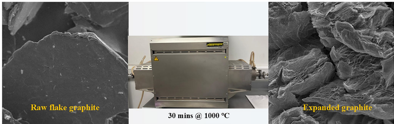
FIGURE 1 | Production of thermally processed expanded graphite.
