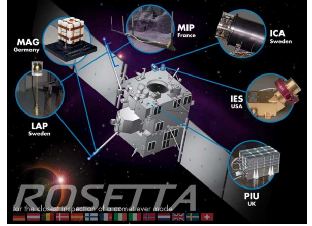
(b) The instruments of the Rosetta Plasma Consortium. Credit: Carr et al. , 2007.
