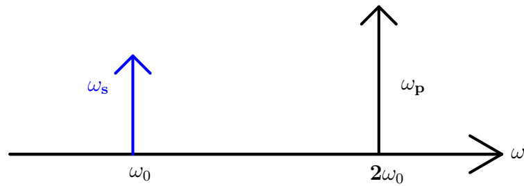
Figure 2.11: Frequency landscape of 3-wave mixing and degenerate process.
