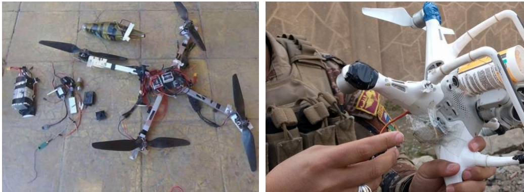
Figure 7. Modified drones of Daesh. Left: home-made quadcopter modified to carry RPG warhead. Right: consumer quadcopter with basic plastic cup holding mechanism for munition release. Photo Source: (B. Watson 2017)
