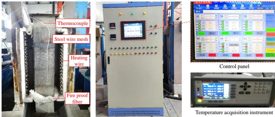
(a) Internal view of the high-temperature electric furnace
