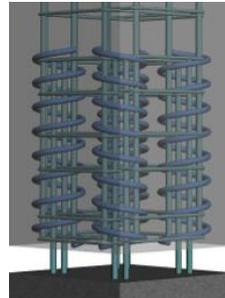
(c) Precast concrete column with cluster reinforcement and constrained grouting-anchor connections
