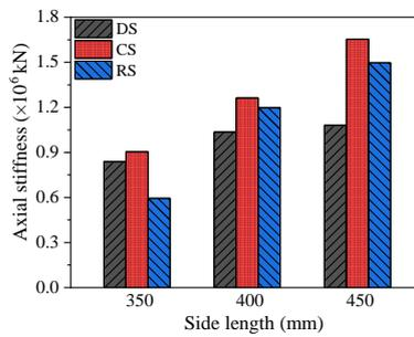
Figure 20 Effect of cross-sectional dimension on axial compressive stiffness
