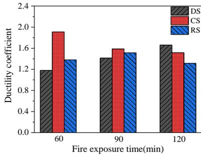
Figure 21 Effect of fire exposure duration on ductility
