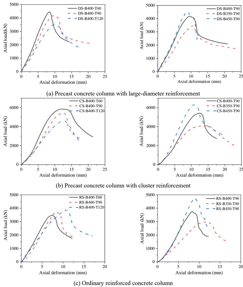
Figure 15 Residual load-deformation response of the test columns
