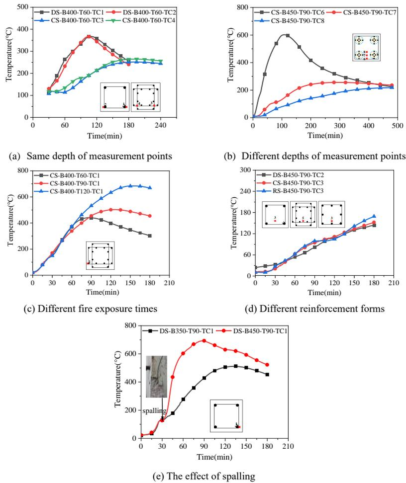
Figure 8 Measured temperatures as a function of time in the tested columns
