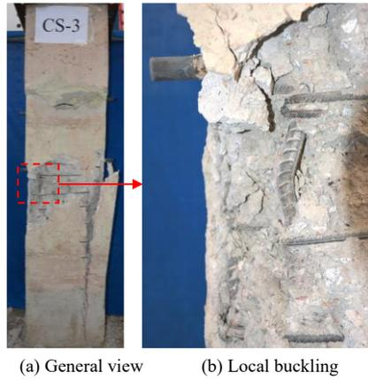
Figure 13 Failure mode of precast concrete column with cluster reinforcement
