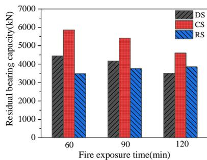
Figure 17 Effect of fire exposure duration on residual load-bearing capacity
