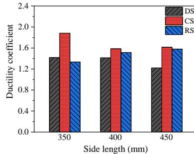
Figure 22 Effect of cross-sectional dimension on ductility
