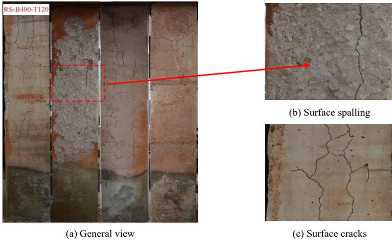
(a) General view (b) Surface spalling (c) Surface cracks
