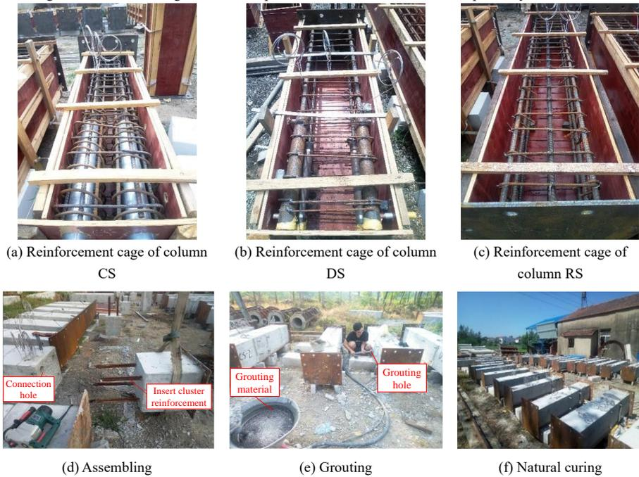
Figure 3 Specimen production process
