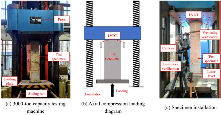
Figure 6 Residual mechanical performance testing setup
