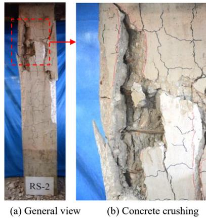
Figure 14 Failure mode of ordinary reinforcement concrete column
