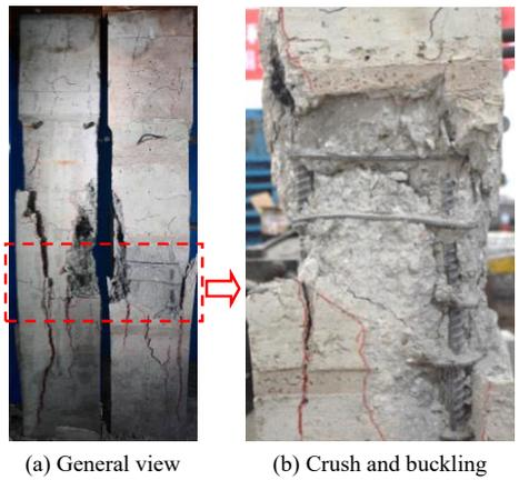
Figure 12 Failure mode of precast concrete column with large-diameter reinforcement
