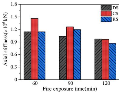
Figure 19 Effect of fire exposure duration on axial compressive stiffness
