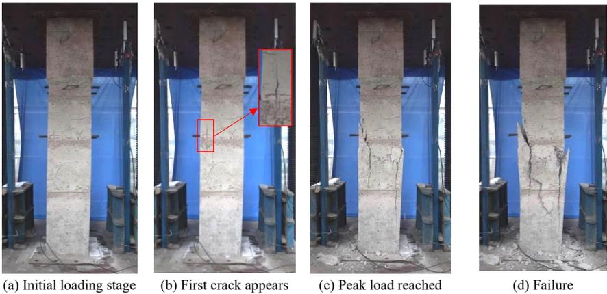
Figure 11 Failure process of precast concrete columns
