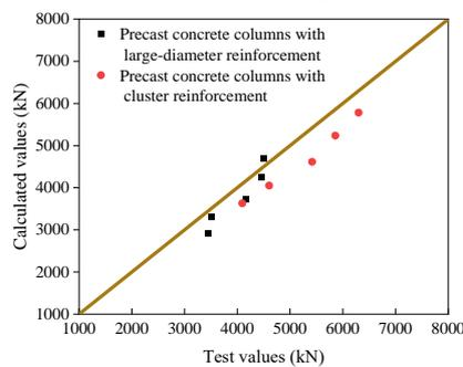
Figure 23 Comparison of calculated and test values of residual load-bearing capacity
