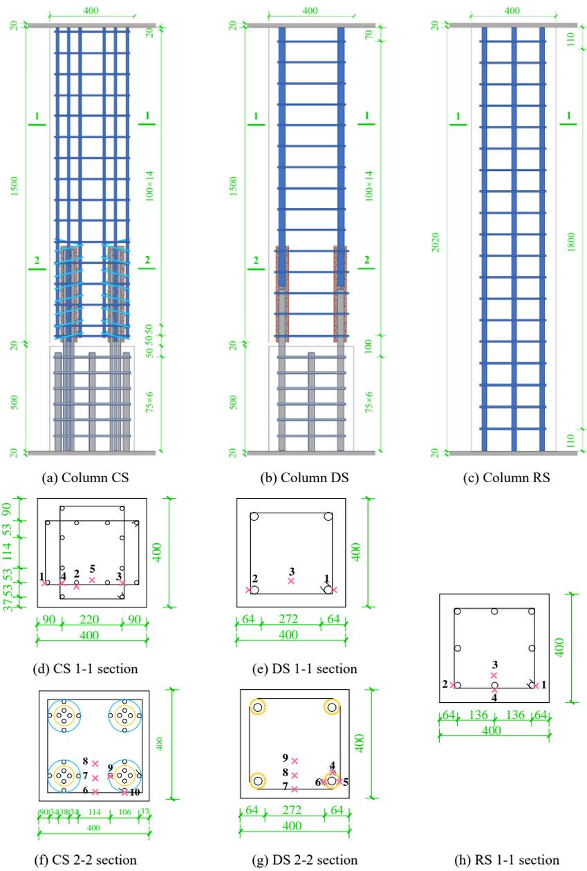
Figure 2 The elevation, cross-section details and thermocouple arrangement of the specimens (mm)
