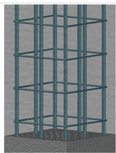
(a) Cast-in-place concrete column with normal reinforcement
