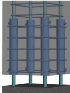
(b) Precast concrete column with large-diameter rebar and sleeve grouting connections
