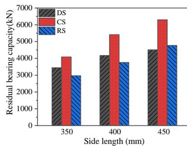
Figure 18 Effect of cross-sectional dimension on residual load-bearing capacity
