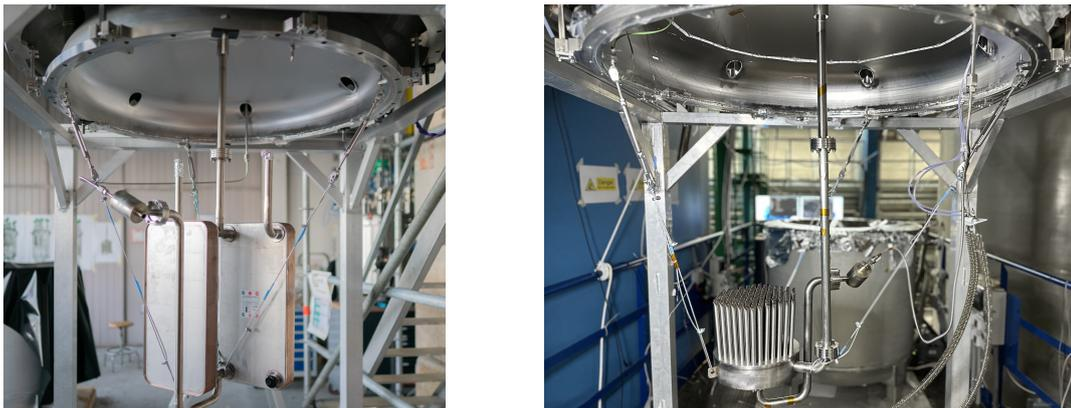
**Figure 5:** Two-phase heat exchanger inside the cryostat to vaporise the return and to condense the supply argon. (Left): Parallel plate geometry. (Right): Multi-tube geometry.
