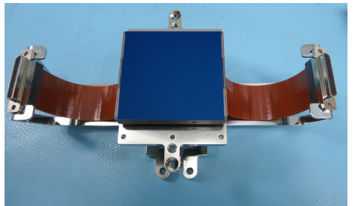
Fig. 8: The CCD273-84 developed specifically for VIS by e2v Technologies.
