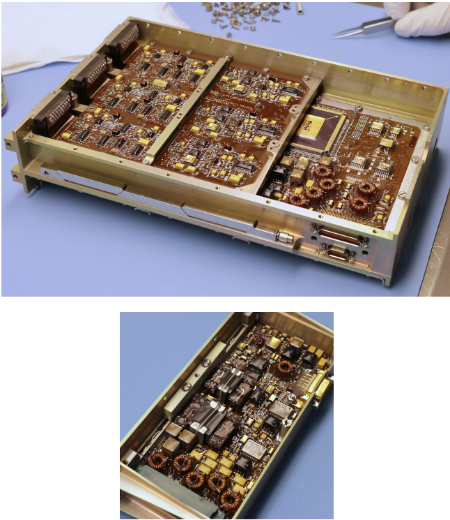
Fig. 13: VIS Readout Electronics ( top ) and Power Supply Unit ( bottom ). The Readout Electronics consists of two double-sided circuit boards containing the twelve analogue channels – three repeating analogue circuits can be seen in the topmost board – with the digital board containing the Field Programmable Gate Array between them and to the rear of the unit. The connectors to the upper flexible connections from the CCDs are at the front of the unit. The Power Supply Unit contains also a tightly populated double-sided circuit board. The planar transformers can be seen on the centre-left of the unit.
