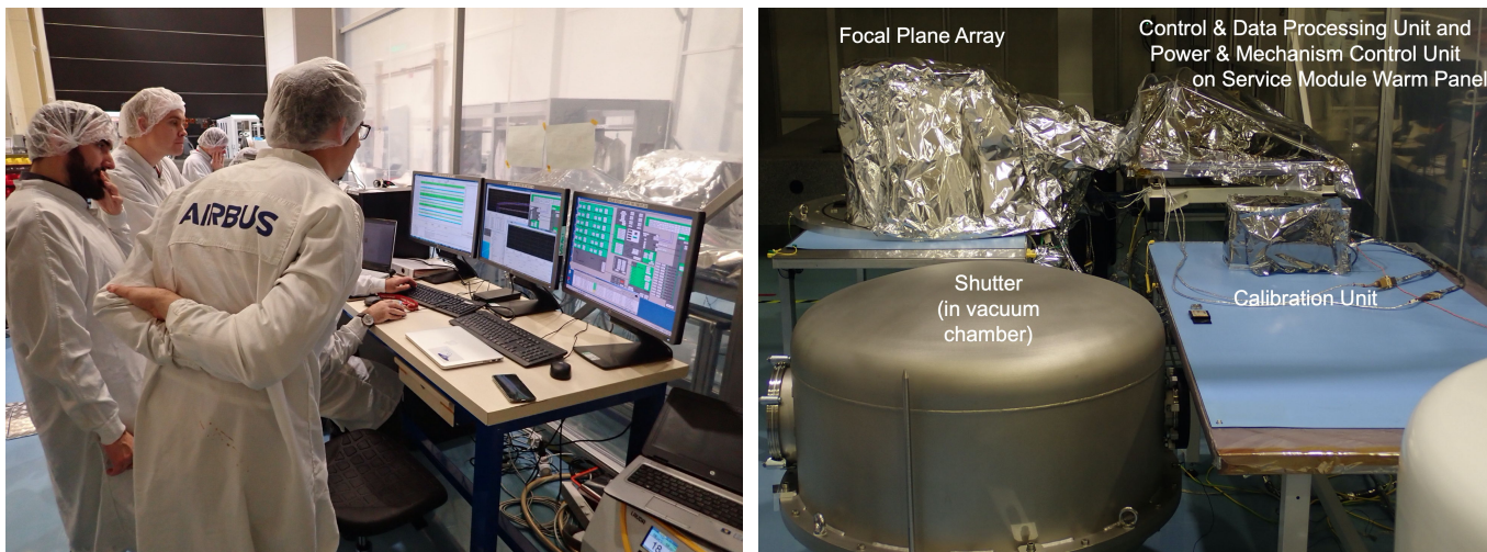
Fig. 17: VIS Flight Model during final testing. This was carried out in an ISO-5 clean area in the Euclid facilities at Airbus (Toulouse); the majority of the Euclid Payload Module is under integration behind the large black shutter. Left : The team inspecting the progress of the Full Functional Test. VIS can be seen foil-covered behind the computer screens. Right : VIS as laid out within the ISO-5 area. The foil-covered Focal Plane Array is in the background connected via 26 harnesses to the Control and Data Processing Unit which is with the Power and Mechanism Control Unit already integrated onto the Service Module Warm Panel (Fig. 6). In the foreground are the foil-covered Calibration Unit and the Shutter in a vacuum chamber. The foil coverings are in place to maintain the stringent levels of cleanliness for VIS, and the vacuum chamber is required to preserve the MoS 2 lubricant during Shutter activation.
