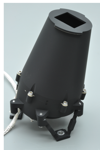
Fig. 13. Flight model of the calibration source NI-CU before integration into NISP. Two supply harnesses can be seen, feeding the nominal and redundant side, respectively, of NI-CU with each 5 LEDs emitting at different wavelengths. Inside the base any LED illuminates the same PTFE reflector patch that in turn directly illuminates the FPA, with a field shaped by a set of five baffles, the last one visible at the top. The full NI-CU height is approximately 150 mm.
