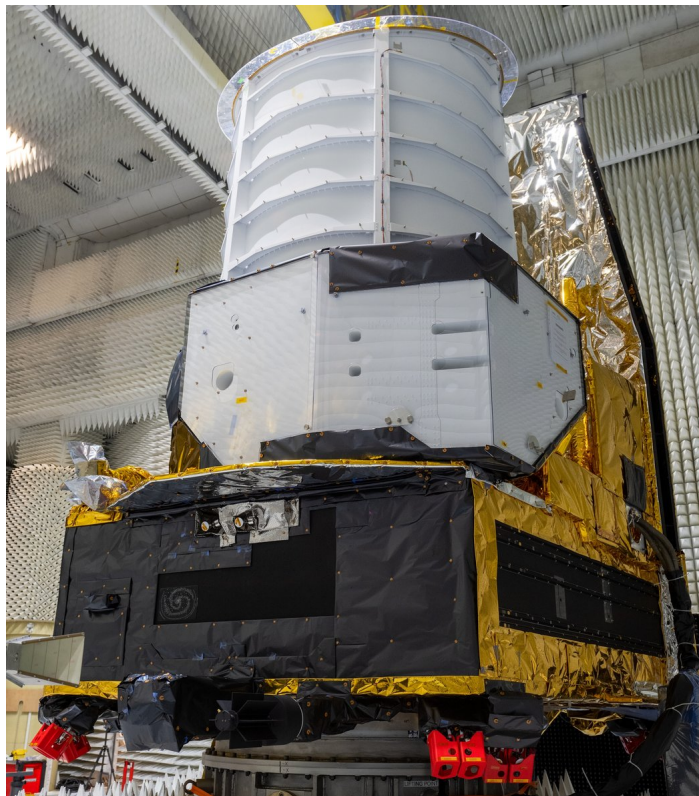
Fig. 5. Left: Overview of the Euclid spacecraft with the principal axes highlighted. Right: The fully assembled spacecraft on February 2023 in the anechoic chamber of Thales Alenia Space in France, after completing final electromagnetic compatibility tests. The side shown here will always face away from the Sun. The large white structure below the cylindrical telescope baffle is the NISP radiator. The hydrazine thrusters still have their protective red covers on. The plaque with the miniaturised fingerprint galaxy created thanks to a collaboration with visual artist Lisa Pettibone and Euclid Consortium members can be seen at the lower left. Figure credit: ESA – M. Pédoussaut.
