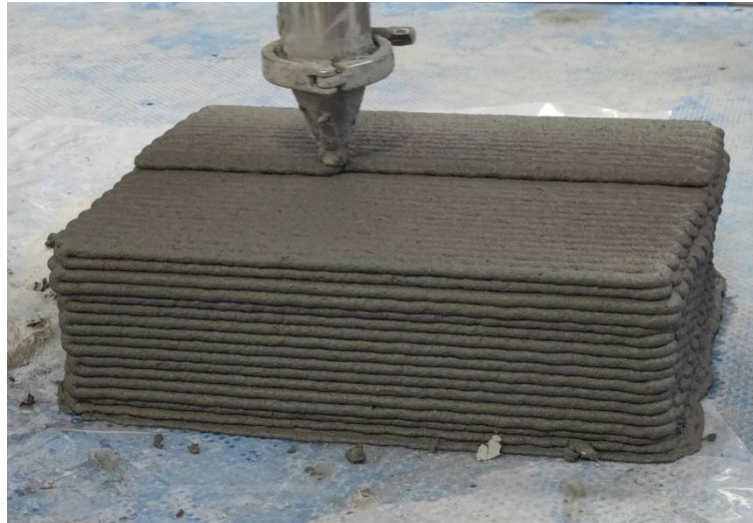
194 195 Figure 5: Printing process of PP fibre reinforced rubberised concrete
