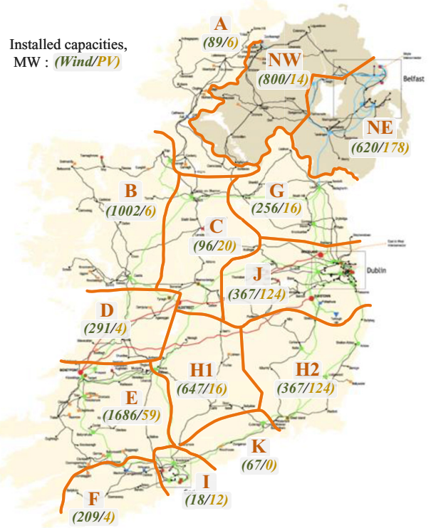
Fig. 2 Ireland transmission network with study areas [13], along with installed wind and PV capacities for 2028 scenario.
