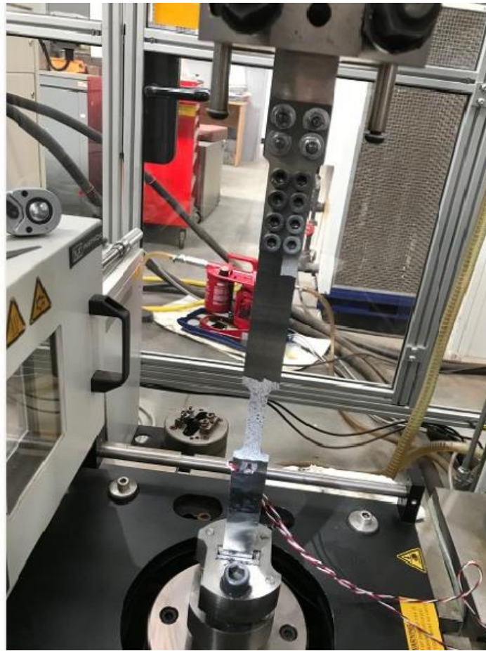
Figure 3-7 Instron machine with sample sprayed with speckle set-up for testing.
