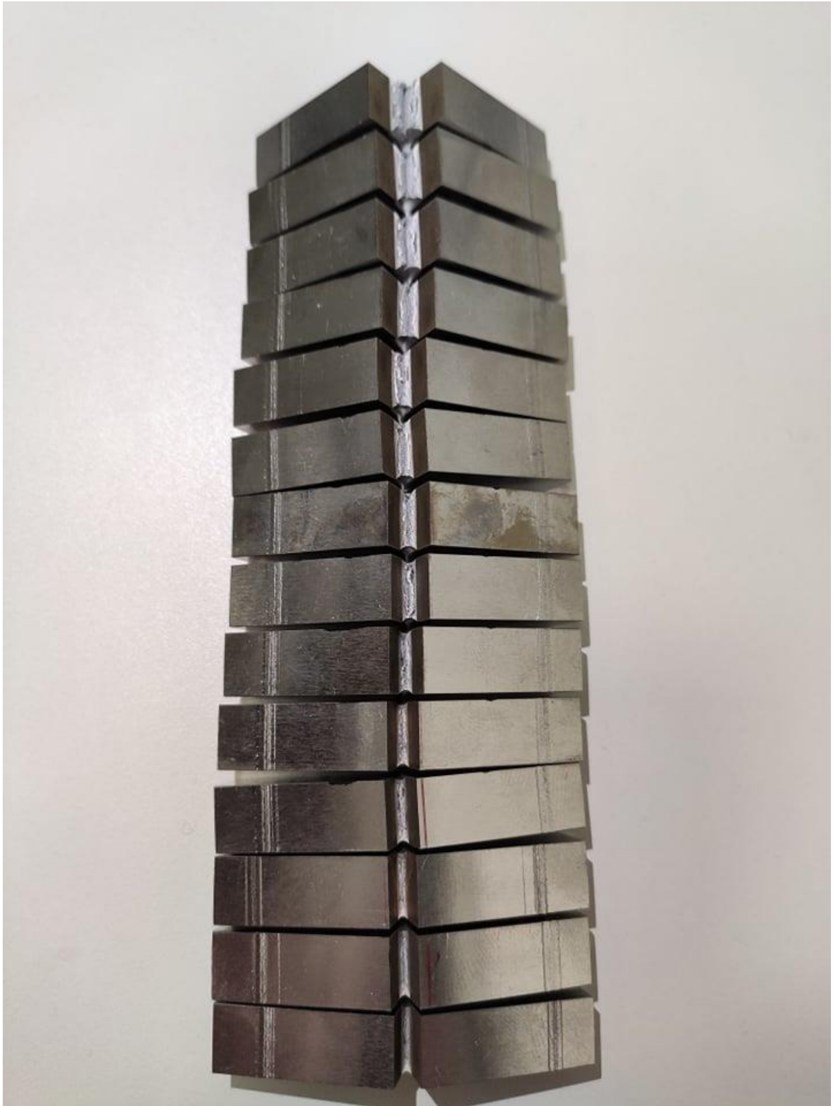
Figure A-2 Fractured notch of impact drop weight test samples.
