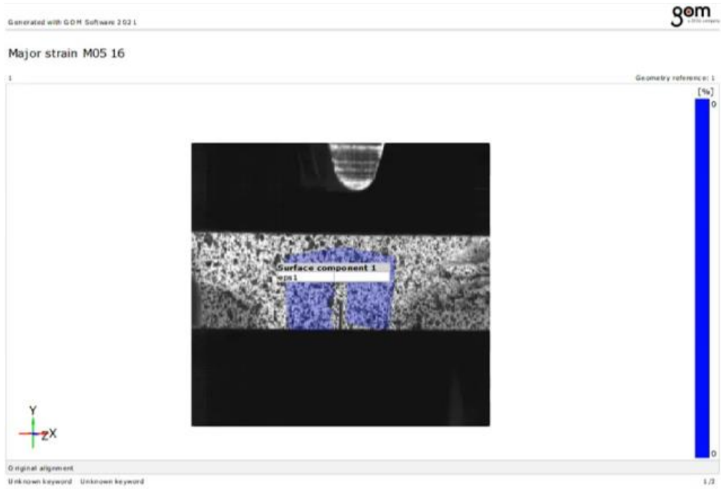
Figure 3-25 Three bend sample with speckle pattern for fracture toughness test
