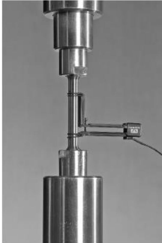
Figure 3-5 A tensile test set up showing the extensometer across the gauge on round specimen (© TWI)
