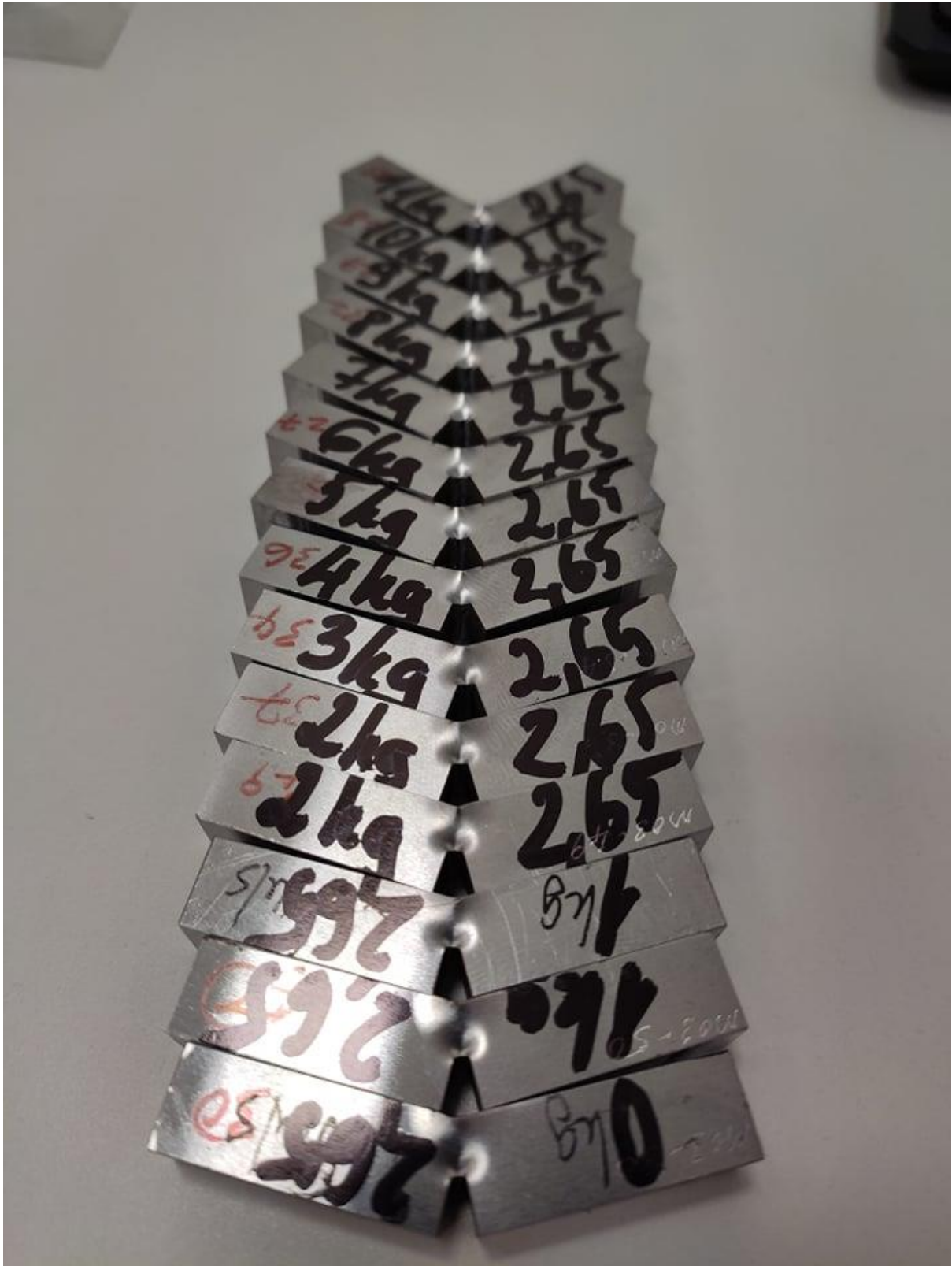
Figure A-1 Impact drop weight tested samples showing the level of crack extension
