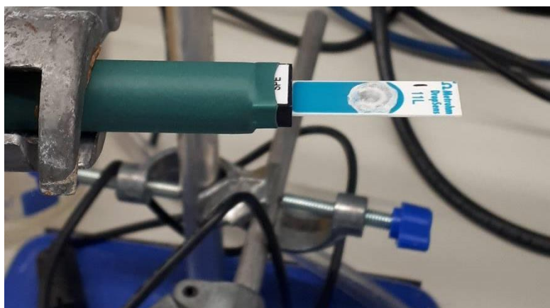
Figure 5.20: SPE setup for spot test on ferrocyanide-KOH film SPE D1.
