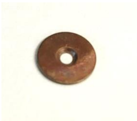
Figure 5.5.3 - Copper ring working electrode, post-analysis corrosion.
