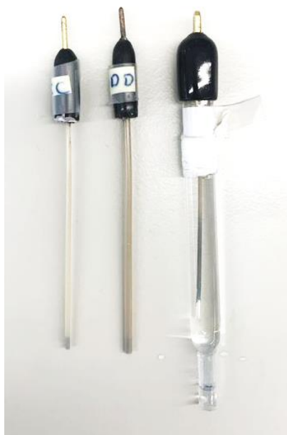
Figure 5.5.2 - Comparison of 'leak-free' \mu Ag/AgCl (left 1 mm O.D., middle 1.6 mm O.D. Innovative Instruments Inc., USA) with conventional, standard Ag/AgCl electrode (right, IJ Cambria, UK). Major difference in size allows flexibility of design with 'leak-free' electrodes, but promised longevity was not met for these experiments.
