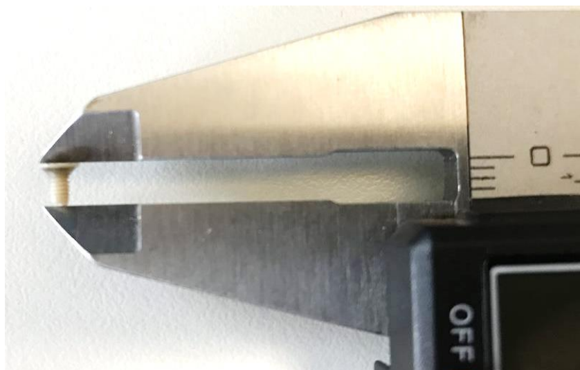
Figure 5.5.4 - Flow through retaining screw size 4 mm.
