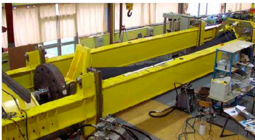
Figure 18. Combined bending fatigue + tension using a test bench (Courtesy: Rampi et al. 2006) (This figure is available in colour online).
