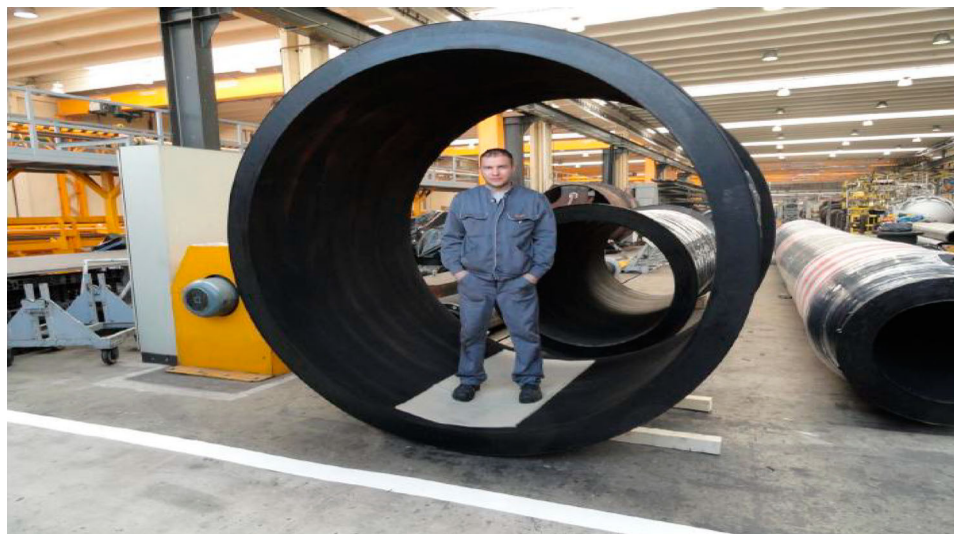
Figure 2. The extreme size of dredging hoses compared to floating hoses (Courtesy: Antal et al. 2012; Adapted with permission of Germa Hornsby of Continental Dunlop Oil & Marine) (This figure is available in colour online).
