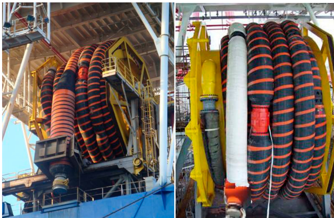
Figure 9. Two hose systems showing reels, reeling hoses, marine breakaway coupling (MBC) and Hose End Valve (HEV) (This figure is available in colour online).
