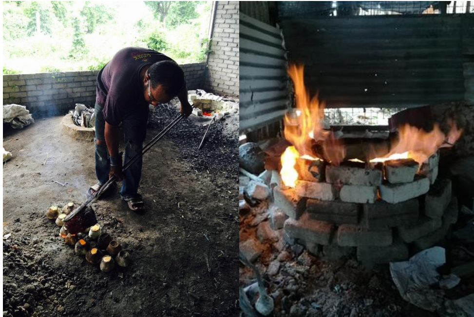
Figure 4.9: Field observations – pouring molten brass and the dewaxing process
