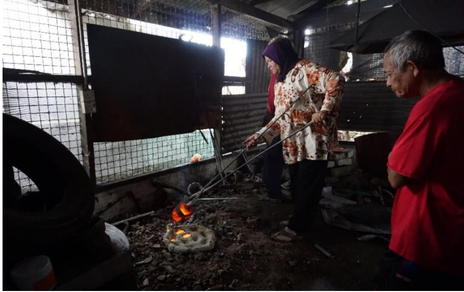
Figure 5.8: Wife of artisan is pouring molten brass into the clay mould
