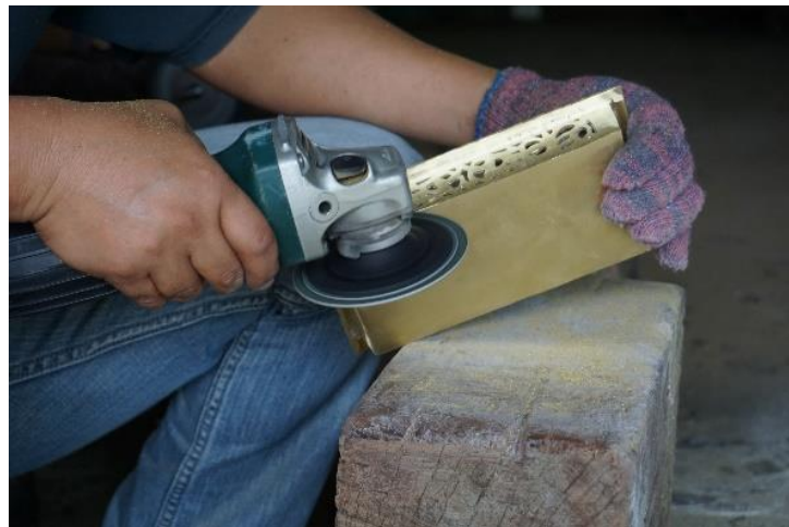
Figure 5.16: Grinding process to remove rough edges using modern tools.
