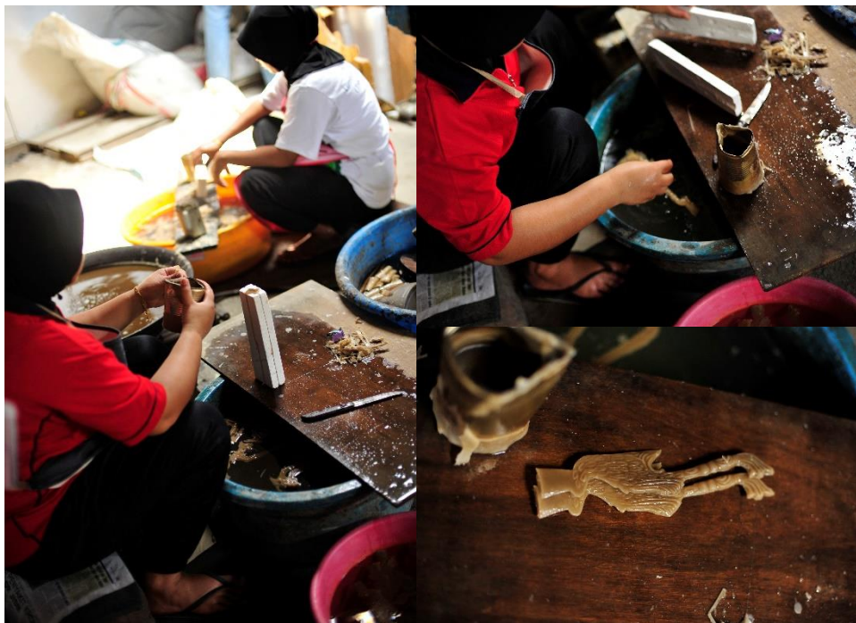
Figure 5.9: Women workers in the production process during the making of wax patterns (photo courtesy of Terengganu State Museum)
