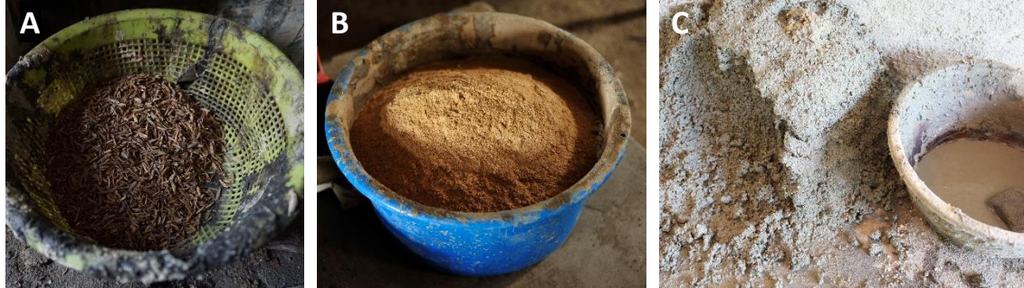
Figure 5.16: A) Rice husk, B) Sand and C) Mixture of clay, sand and water
