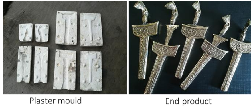
Figure 6.12: Plaster mould for wax pattern of keris (Malay dagger) and its end product
