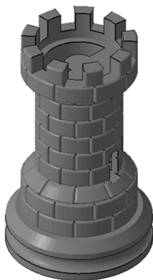
Fig. 6 Chess rook containing 93,930 triangles, dimensions: 31.75 \times 31.75 \times 53.15 mm
