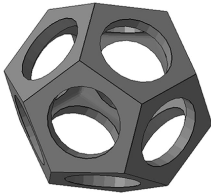
Fig. 10 Dodecahedra model consisting of 2074 triangles, 157.81 \times 133.62 \times 165.15 mm
