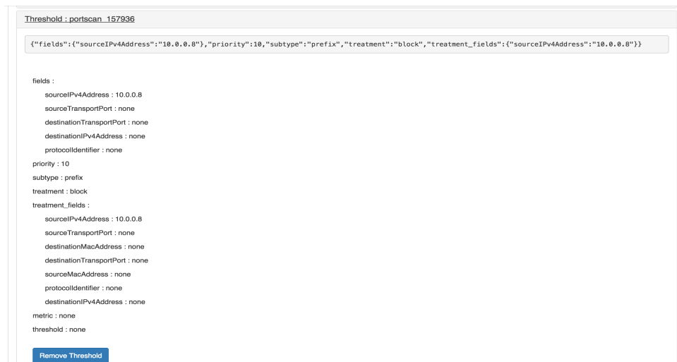
Figure 1: Port scan threshold details
