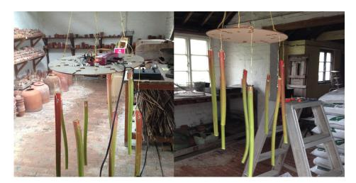
**Figure 5.15:** A Rhubaphone prototype designed to look like a wind chime. This iteration uses a Raspberry Pi, Arduino and sensor.
