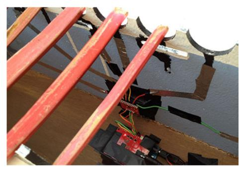
Figure 5.14: Electronics and aluminium tape inside the first prototype
