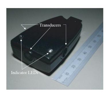
The Relate Dongles provide finegrained relative position information to co-located devices on the basis of peer-to-peer sensing, to directly establish their spatial relationships, without need for infrastructure in their environment.
