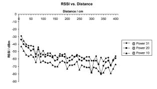
Figure 5 – RSSI between two IEEE 802.15.4 nodes with 9db attenuation on transmitter. Standard deviation: mean 8.16dBm, max 14.66dBm, min 6.11dBm
