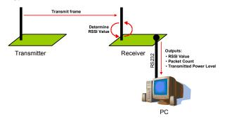
Figure 2 - Experiment Configuration
