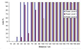
Figure 6 – Packet loss observed between two IEEE 802.15.4 nodes with 9db attenuation on transmitter.
