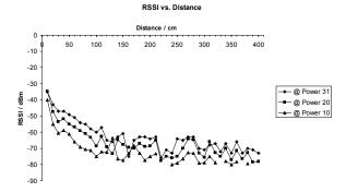
Figure 7 – RSSI between two IEEE 802.15.4 nodes with 9db attenuation on transmitter and fixed LNA gain on receiver. Std. dev.: mean 4.52dBm, max 7.06dBm, min 2.20dBm
