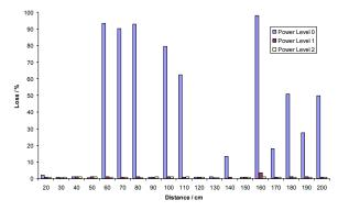
Figure 4 – Packet loss observed between two IEEE 802.15.4 nodes with factory default setting.
