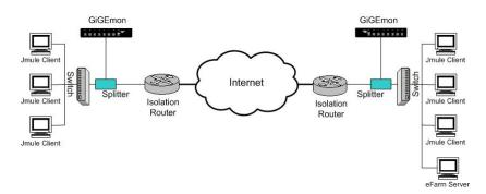
Figure 3: Experimental Packet Capture Environment
