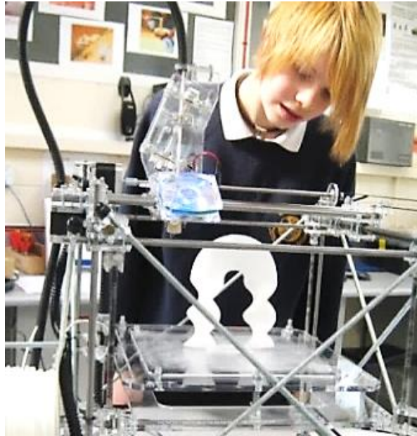
Figure 2.11: Entry Level Desktop AM machine - RepRap ® [128].
