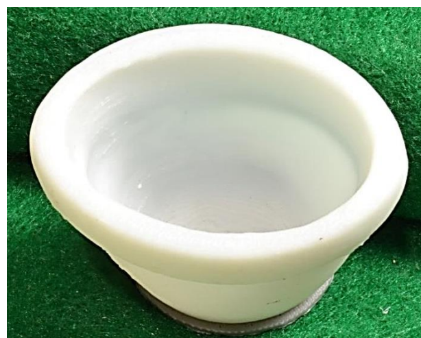
Figure 8.52: Repaired FDM model of Vase.
