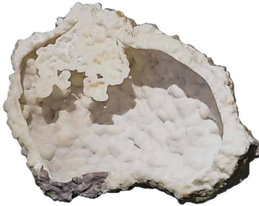
Figure 8.61: Hollow underside of SLS concrete mix replica.
