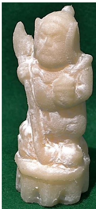
Figure 8.48: Full size Warrior SLS model with residual powder.
