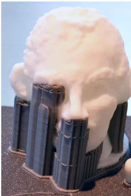
Figure 8.25: The FDM model head with structure supports.
