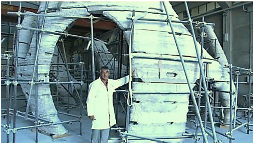
Figure 8.8: Enrico Dini of Monolite UK with Radiolaria - the biggest structure ever built by the D-Shape 3D printer [237].
