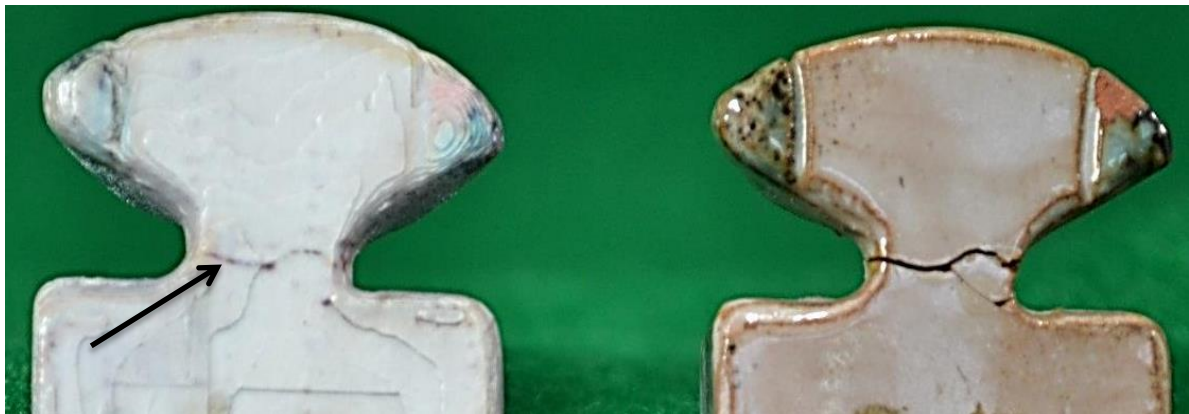
Figure 8.17: Left hand figurine with hair line printed crack visible.
