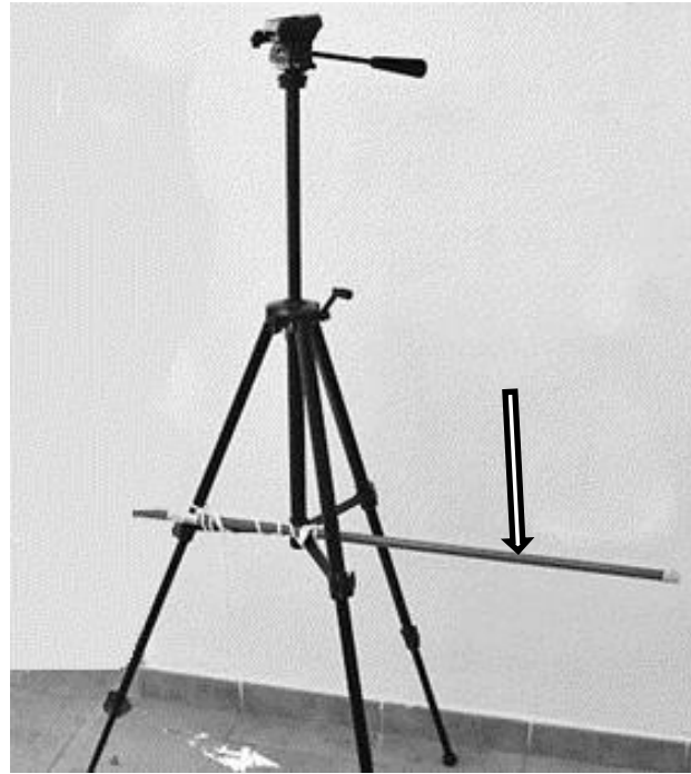
Figure 3.16: Use of pole to control radial distance of camera position.
