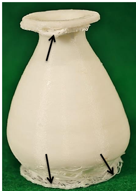
Figure 8.38: Incomplete FDM model showing detached filaments.
