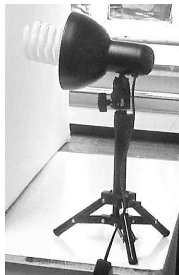
Figure 3.19: Single bulb 45W floodlight.
