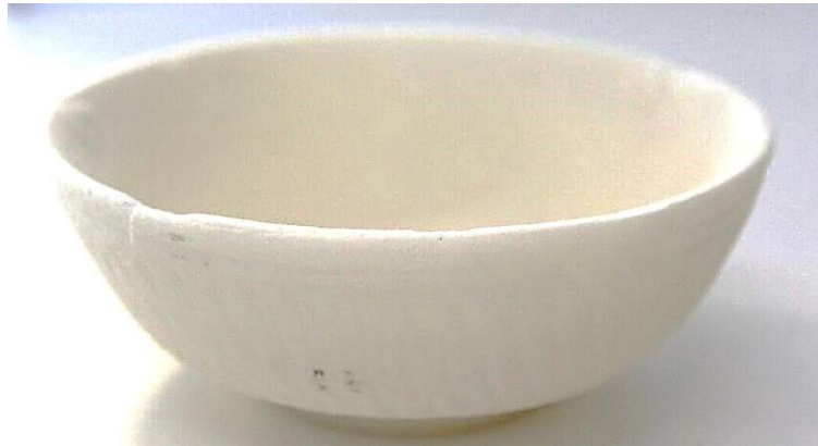
Figure 8.34: The digitally repaired and SLS fabricated Egyptian Bowl.
