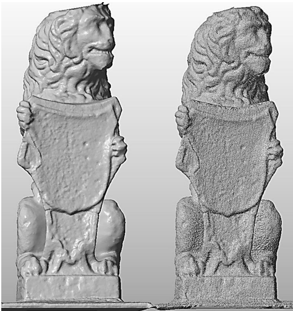
Figure 7.13: Screen shot from StudioPro ® Imported from: Left – 123D Catch ® Right – PhotoScan Pro ® .
