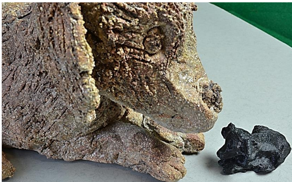
Figure 8.3: Miniature FDM black dog – 50mm long x 20mm high seen alongside original clay dog.
