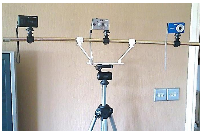
Figure 3.11: Curved pipe supporting three compact cameras.
