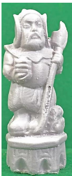
Figure 4.80: Ultimaker 250 \mu m model.
