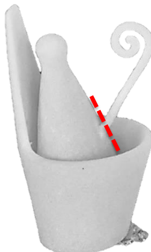
Figure 6.39: FDM printed model - version 1 – without support bar – unpainted.
