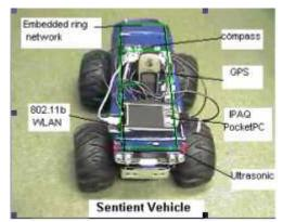
Figure 2 – A top view of sentient vehicle
