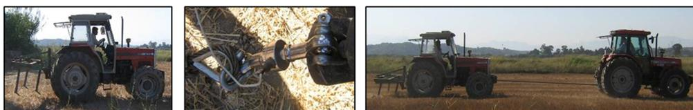
**Figure 2.** Subsoiler-tractor connections, dynamometer and experimental study.
