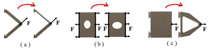
Figure 8. Structural optimization: size (a), shape (b) and topological optimization (c).
