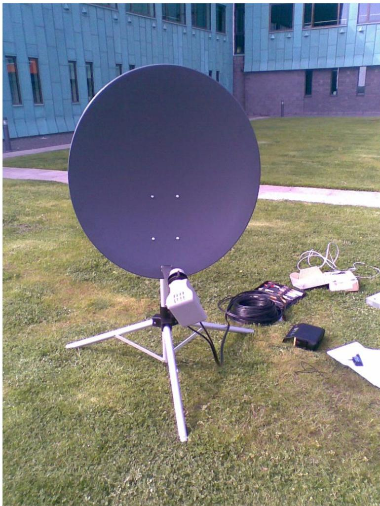
Figure 8 : Astra2Connect equipment being fully set up (front side of dish)
