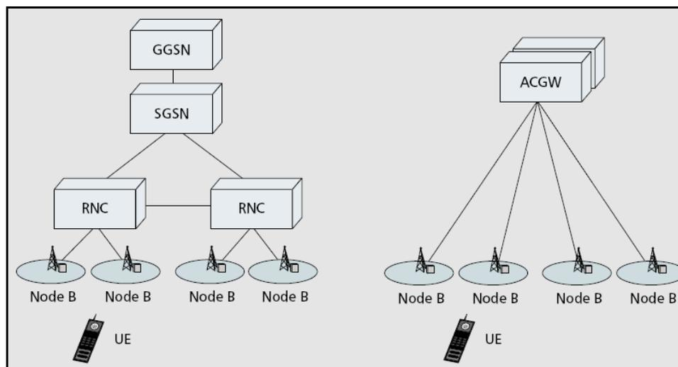
Figure 1 : 3GPP Release 6 Architecture (left) and Evolved 3G Access Architecture (right) [11]
