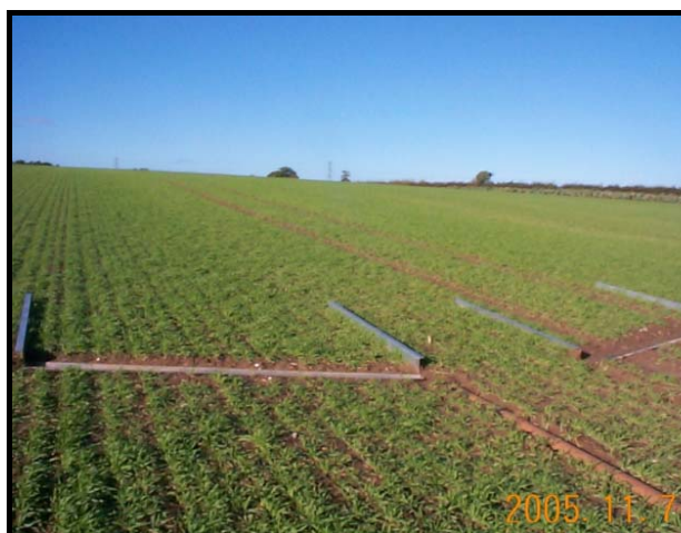
Plate 1a. Layout of hillslope monitoring equipment. Runoff from the upslope monitoring area was collected by plastic or metal gutters which channelled runoff into the piping.
