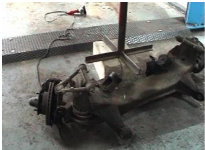
Fig. 14. The subframe removed
